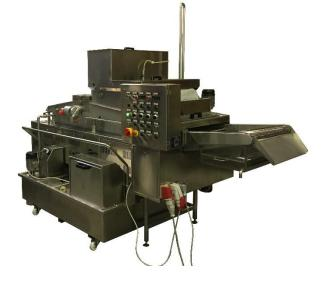
The filtering system guarantees excellent cleaning, long life and extreme practicality. The oil pumped from the fryer's tank to the paper filter, is filtered by a special food paper (suitable for use up to a temperature of 200 ° C) which retains cooking residues, flour, and small particles, leaving pass the clean oil, which, by choice, falls back into the fryer tank or into the oil top-up tank.
